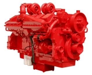
1800 RPM up to 5000 ft. (1500 m) and 104° F (40 °C) without power deration. 1500 RPM up to 5000 ft. (1500 m) and 104 ° F (40 °C) without power deration. For sustained operation above these conditions, derate by 4% per 1,000 ft.(300 m), and 1% per 10 ° F (2% per 11 °C).
