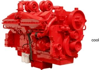
The engine may be operated at : 1800 RPM up to 5000 ft. (1500 m) and 104° F (40  $^{\circ}$ C) without power deration. 1500 RPM up to 5000 ft. (1500 m) and 104  $^{\circ}$  F (40  $^{\circ}$ C) without power deration. For sustained operation above these conditions, derate by 4% per 1,000 ft.(300 m), and 1% per 10 ° F (2% per 11 °C).
