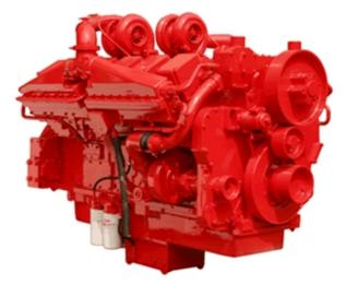
1800 RPM up to 5000 ft. (1525 m) and 104° F (40  $^{\circ}$ C) without power deration. 1500 RPM up to 5000 ft. (1525 m) and 104  $^{\circ}$  F (40  $^{\circ}$ C) without power deration. For sustained operation above these conditions, derate by 4% per 1,000 ft.(300 m), and 1% per 10  $^{\circ}$  F (2% per 11  $^{\circ}$ C).
