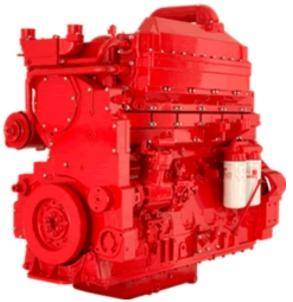
1800 RPM up to 5000 ft. (1500 m) and 104° F (40  $^{\circ}$ C) without power deration. 1500 RPM up to7500 ft. (2280 m) and 104 ° F (40  $^{\circ}$ C) without power deration. For sustained operation above these conditions, derate by 4% per 1,000 ft.(300 m), and 1% per 10 ° F (2% per 11  $^{\circ}$ C).
